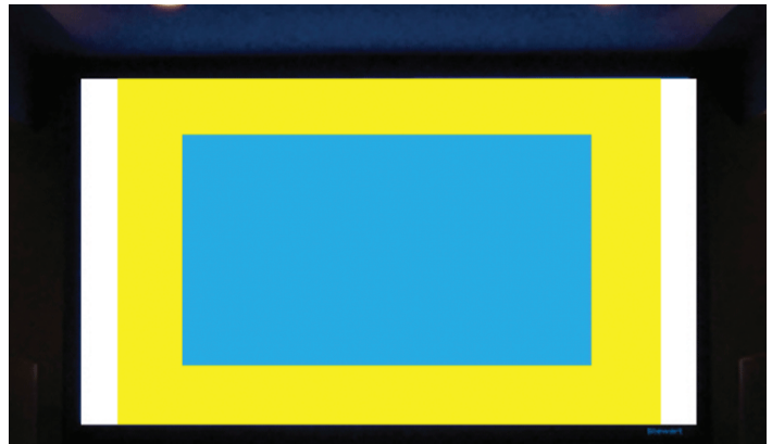
The white area represents the 2.0 native screen canvas (2.0:1), with the yellow area representing a 1.78:1 aspect ratio in the 2.0 solution, and the blue representing a constant height 1.33:1 image area. The Director's Choice 2.0 1.78:1 image area is 39%* larger than the constant height's image area.
